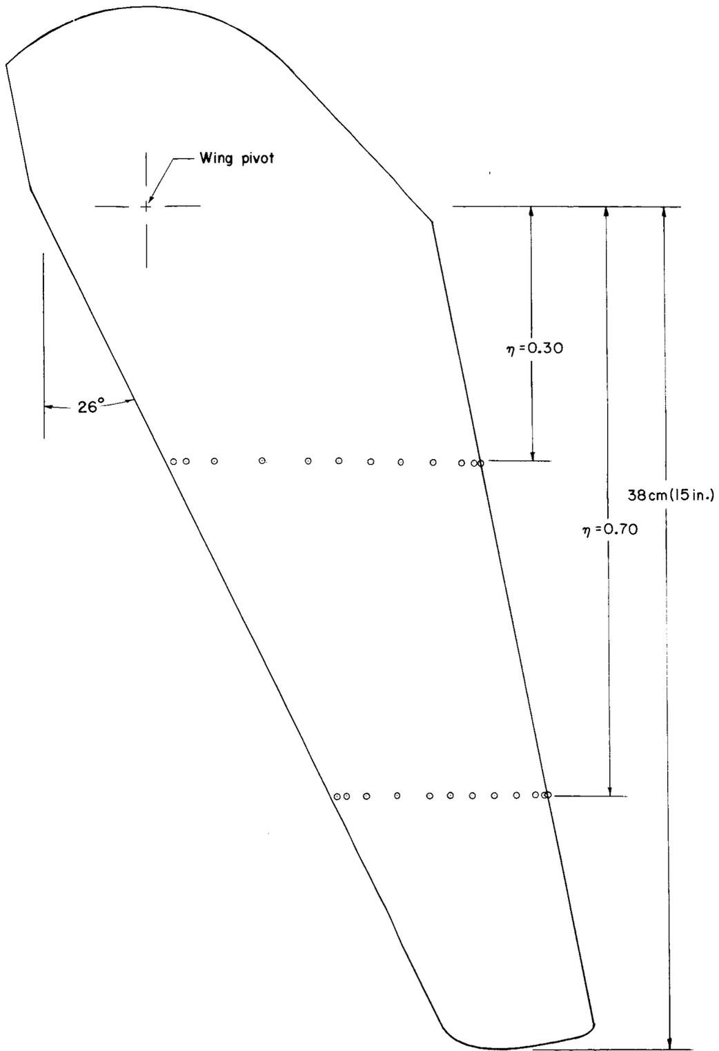
Figure 5.- Wing planform showing pressure orifice locations.
